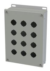
Saginaw pushbutton enclosure, 12 holes, 30mm, NEMA 4/12/13, 12 x 9 x 3in (HxWxD), wall mount, carbon steel, ANSI 61 gray, powder coat finish, screw cover.
