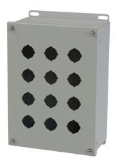
Saginaw pushbutton enclosure, 12 holes, 30mm, NEMA 4/12/13, 12 x 9 x 5in (HxWxD), wall mount, carbon steel, ANSI 61 gray, powder coat finish, screw cover.
