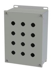
Saginaw pushbutton enclosure, 12 holes, 22mm, NEMA 4/12/13, 12 x 9 x 5in (HxWxD), wall mount, carbon steel, ANSI 61 gray, powder coat finish, screw cover.
