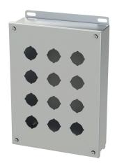
Saginaw pushbutton enclosure, 12 holes, 30mm, NEMA 4/4X/12/13, 12 x 9 x 3in (HxWxD), wall mount, 316L stainless steel, #4 brush finish, screw cover.
