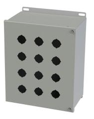
Saginaw pushbutton enclosure, 12 holes, 30mm, NEMA 4/12/13, 12 x 10 x 6in (HxWxD), wall mount, carbon steel, ANSI 61 gray, powder coat finish, hinged screw cover.
