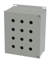
Saginaw pushbutton enclosure, 12 holes, 22mm, NEMA 4/12/13,  $12 \times 10 \times 6$ in (HxWxD), wall mount, carbon steel, ANSI 61 gray, powder coat finish, hinged screw cover.
