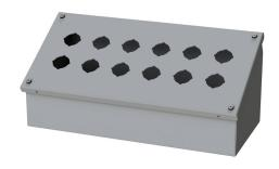
Saginaw pushbutton consolet, 12 holes, 30mm, NEMA 4/12/13, 7 x 16 x 7in (HxWxD), wall mount, carbon steel, ANSI 61 gray, powder coat finish, screw cover, purchase subpanel separately.
