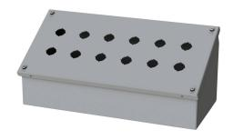
Saginaw pushbutton consolet, 12 holes, 22mm, NEMA 4/12/13, 7 x 16 x 7in (HxWxD), wall mount, carbon steel, ANSI 61 gray, powder coat finish, screw cover, purchase subpanel separately.
