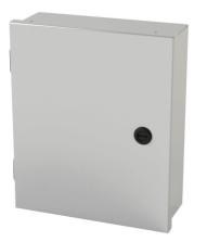
Saginaw enclosure, NEMA 1,  $12 \times 10 \times 4$  in (HxWxD), wall mount, carbon steel, ANSI 61 gray, powder coat finish, single-door, 1/4-turn semi-flush latch.
