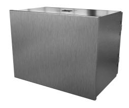
Saginaw HMI Enclosure, NEMA 3R/4/4X/12/13, 12 x 16 x 10in (HxWxD), suspension or pedestal mount, dual access, 304 stainless steel, #4 brush finish, screw cover front, single door rear, 1/4-turn semi-flush latch.
