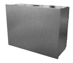
Saginaw HMI Enclosure, NEMA 3R/4/4X/12/13, 12 x 16 x 6in (HxWxD), suspension or pedestal mount, dual access, 304 stainless steel, #4 brush finish, screw cover front, single door rear, 1/4-turn semi-flush latch.
