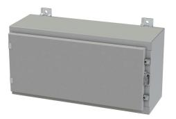
Saginaw enclosure, NEMA 3R/4/12/13,  $12 \times 24 \times 8in$  (HxWxD), wall mount, carbon steel, ANSI 61 gray, powder coat finish, single-door, plated steel clamps, padlock hasp and staple.
