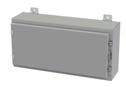
Saginaw enclosure, NEMA 3R/4/12/13, 12 x 24 x 6in (HxWxD), wall mount, carbon steel, ANSI 61 gray, powder coat finish, single-door, plated steel clamps, padlock hasp and staple.
