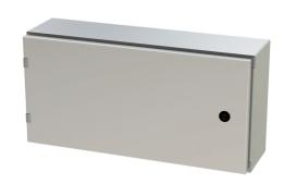
Saginaw Enviroline series enclosure, NEMA 3R/4/4X/12/13, 12 x 24 x 6in (HxWxD), wall mount, 304 stainless steel, #4 brush finish, single-door, 1/4-turn semi-flush latch.
