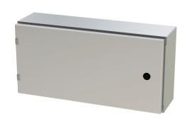
Saginaw Enviroline series enclosure, NEMA 3R/4/4X/12/13,  $12 \times 24 \times 6$  in (HxWxD), wall mount, 304 stainless steel, #4 brush finish, single-door, 1/4-turn semi-flush latch.
