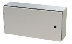
Saginaw Enviroline series enclosure, NEMA 3R/4/4X/12/13,  $12 \times 24 \times 6in$  (HxWxD), wall mount, 316L stainless steel, #4 brush finish, single-door, 1/4-turn semi-flush latch.
