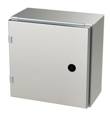
Saginaw Enviroline series enclosure, NEMA 3R/4/4X/12/13,  $12 \times 12 \times 6$  in (HxWxD), wall mount, 304 stainless steel, #4 brush finish, single-door, 1/4-turn semi-flush latch.
