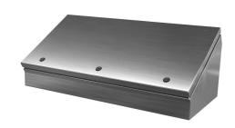
Saginaw operator consolet, NEMA 3R/4/4X/12/13, 12 x 24 x 9in (HxWxD), desktop or pedestal mount, 304 stainless steel, #4 brush finish, single-door, 1/4-turn semi-flush latch.
