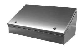
Saginaw operator consolet, NEMA 3R/4/4X/12/13,  $12 \times 20 \times 9$ in (HxWxD), desktop or pedestal mount, 304 stainless steel, #4 brush finish, single-door, 1/4-turn semi-flush latch.
