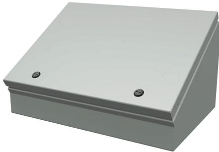
Saginaw operator console, NEMA 3R/4/12/13, 12 x 16 x 9in (HxWxD), desktop or pedestal mount, carbon steel, ANSI 61 gray, powder coat finish, single-door, 1/4-turn semi-flush latch.
