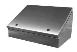
Saginaw operator consolet, NEMA 3R/4/4X/12/13, 12 x 16 x 9in (HxWxD), desktop or pedestal mount, 304 stainless steel, #4 brush finish, single-door, 1/4-turn semi-flush latch.
