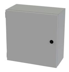
Saginaw Enviroline Junction series enclosure, NEMA 3R/4/12/13, 12 x 12 x 6in (HxWxD), wall mount, carbon steel, ANSI 61 gray, powder coat finish, single-door, 1/4-turn semi-flush latch.
