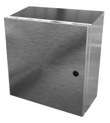
Saginaw Enviroline Junction series enclosure, slope top, NEMA 3R/4/4X/12/13,  $12 \times 12 \times 6in$  (HxWxD), wall mount, 304 stainless steel, #4 brush finish, single-door, 1/4-turn semi-flush latch.
