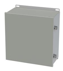
Saginaw enclosure, NEMA 3R/4/12/13, 12 x 12 x 6in (HxWxD), wall mount, carbon steel, ANSI 61 gray, powder coat finish, single-door, stainless steel clamps.
