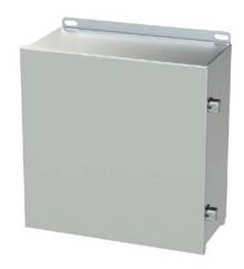
Saginaw enclosure, NEMA 3R/4/4X/12/13,  $12 \times 12 \times 6$ in (HxWxD), wall mount, 304 stainless steel, #4 brush finish, single-door, stainless steel clamps.
