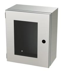
Saginaw Enviroline Junction series enclosure, NEMA 3R/4/4X/12/13,  $12 \times 10 \times 6$  in (HxWxD), wall mount, 316L stainless steel, #4 brush finish, single-door, 1/4-turn semi-flush latch, polycarbonate window.
