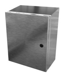
Saginaw Enviroline Junction series enclosure, slope top, NEMA 3R/4/4X/12/13,  $12 \times 10 \times 6$ in (HxWxD), wall mount, 304 stainless steel, #4 brush finish, single-door, 1/4-turn semi-flush latch.
