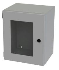
Saginaw Enviroline Junction series enclosure, NEMA 3R/4/12/13, 12 x 10 x 8in (HxWxD), wall mount, carbon steel, ANSI 61 gray, powder coat finish, single-door, 1/4-turn semi-flush latch, polycarbonate window.
