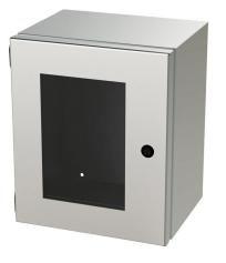
Saginaw Enviroline Junction series enclosure, NEMA 3R/4/4X/12/13, 12 x 10 x 8in (HxWxD), wall mount, 304 stainless steel, #4 brush finish, single-door, 1/4-turn semi-flush latch, polycarbonate window.
