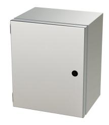
Saginaw Enviroline Junction series enclosure, NEMA 3R/4/4X/12/13,  $12 \times 10 \times 8$  in (HxWxD), wall mount, 304 stainless steel, #4 brush finish, single-door, 1/4-turn semi-flush latch.
