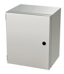
Saginaw Enviroline Junction series enclosure, NEMA 3R/4/4X/12/13, 12 x 10 x 8in (HxWxD), wall mount, 316L stainless steel, #4 brush finish, single-door, 1/4-turn semi-flush latch.
