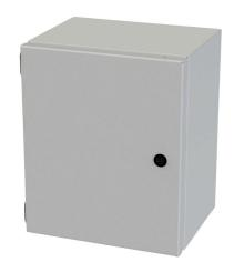
Saginaw Enviroline Junction series enclosure, NEMA 3R/4/12/13,  $12 \times 10 \times 8$  in (HxWxD), wall mount, carbon steel, RAL 7035 light gray, powder coat finish, single-door, 1/4-turn semi-flush latch.
