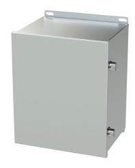
Saginaw enclosure, NEMA 3R/4/4X/12/13, 12 x 10 x 8in (HxWxD), wall mount, 316L stainless steel, #4 brush finish, single-door, stainless steel clamps.
