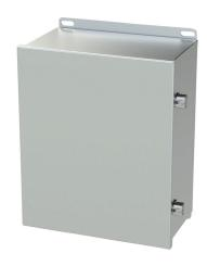
Saginaw enclosure, NEMA 3R/4/4X/12/13,  $12 \times 10 \times 6$ in (HxWxD), wall mount, 304 stainless steel, #4 brush finish, single-door, stainless steel clamps.
