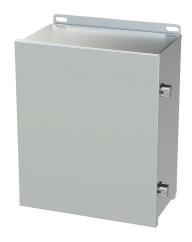
Saginaw enclosure, NEMA 3R/4/4X/12/13, 12 x 10 x 6in (HxWxD), wall mount, 304 stainless steel, #4 brush finish, single-door, stainless steel clamps.
