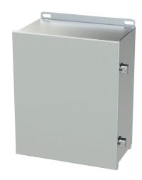
Saginaw enclosure, NEMA 3R/4/4X/12/13, 12 x 10 x 6in (HxWxD), wall mount, 316L stainless steel, #4 brush finish, single-door, stainless steel clamps.
