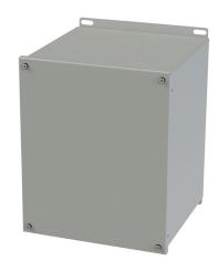
Saginaw enclosure, NEMA 3R/4/12/13, 12 x 10 x 10in (HxWxD), wall mount, carbon steel, ANSI 61 gray, powder coat finish, screw cover.
