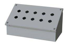
Saginaw pushbutton consolet, 10 holes, 22mm, NEMA 4/12/13,  $7 \times 13 \times 7$ in (HxWxD), wall mount, carbon steel, ANSI 61 gray, powder coat finish, screw cover, purchase subpanel separately.
