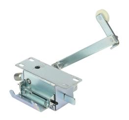
Saginaw mechanical interlock, interlocks the master door on left to the slave door on right. For use with Enviroline two-door enclosures greater than 30in (H) with a center channel between doors.
