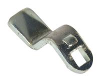
Saginaw 28mm latch cam, replacement, carbon steel, plated zinc finish. For use with Series 14 console top with SCE-MINxxxx miniature 1/4-turn latches.
