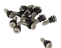
Saginaw cover screw, replacement, #10-32 UNF x 0.625in, Phillips pan head, stainless steel. Nylon retainer included.
