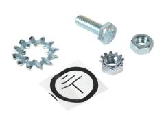
Saginaw ground screw, 1/4-20 UNC x 0.625in, hex head. For use with 3/8-16 subpanel mounts. Hex nut, kep nut, lock washer and grounding label included.
