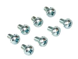
Saginaw subpanel bolt, replacement, 1/4-20 UNC x 0.375in, Phillips pan head, carbon steel, zinc plated finish. Package of 8. Washer included.
