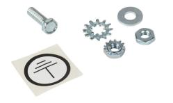
Saginaw ground screw, #10-32 UNF x 0.625in, hex head. For use with #10-32 subpanel mounts. Hex nut, kep nut, flat washer, lock washer and grounding label included.
