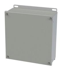
Saginaw enclosure, NEMA 3R/4/12/13, 10 x 10 x 4in (HxWxD), wall mount, carbon steel, ANSI 61 gray, powder coat finish, screw cover.
