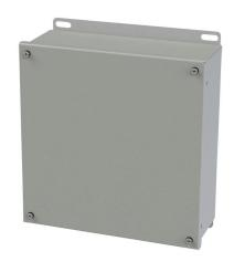
Saginaw enclosure, NEMA 3R/4/12/13, 10 x 10 x 4in (HxWxD), wall mount, carbon steel, ANSI 61 gray, powder coat finish, screw cover.
