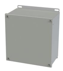
Saginaw enclosure, NEMA 3R/4/12/13, 10 x 10 x 6in (HxWxD), wall mount, carbon steel, ANSI 61 gray, powder coat finish, screw cover.
