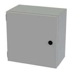
Saginaw Enviroline Junction series enclosure, NEMA 3R/4/12/13,  $10 \times 10 \times 6$  in (HxWxD), wall mount, carbon steel, ANSI 61 gray, powder coat finish, single-door, 1/4-turn semi-flush latch.
