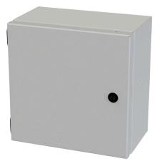
Saginaw Enviroline Junction series enclosure, NEMA 3R/4/12/13,  $10 \times 10 \times 6$  in (HxWxD), wall mount, carbon steel, RAL 7035 light gray, powder coat finish, single-door, 1/4-turn semi-flush latch.
