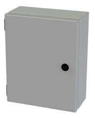
Saginaw Enviroline Junction series enclosure, NEMA 3R/4/12/13, 10 x 8 x 4in (HxWxD), wall mount, carbon steel, ANSI 61 gray, powder coat finish, single-door, 1/4-turn semi-flush latch.
