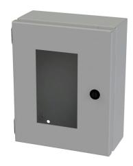
Saginaw Enviroline Junction series enclosure, NEMA 3R/4/12/13,  $10 \times 8 \times 4$  in (HxWxD), wall mount, carbon steel, ANSI 61 gray, powder coat finish, single-door, 1/4-turn semi-flush latch, polycarbonate window.
