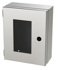
Saginaw Enviroline Junction series enclosure, NEMA 3R/4/4X/12/13, 10 x 8 x 4in (HxWxD), wall mount, 304 stainless steel, #4 brush finish, single-door, 1/4-turn semi-flush latch, polycarbonate window.
