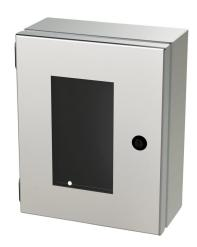
Saginaw Enviroline Junction series enclosure, NEMA 3R/4/4X/12/13,  $10 \times 8 \times 4$  in (HxWxD), wall mount, 316L stainless steel, #4 brush finish, single-door, 1/4-turn semi-flush latch, polycarbonate window.
